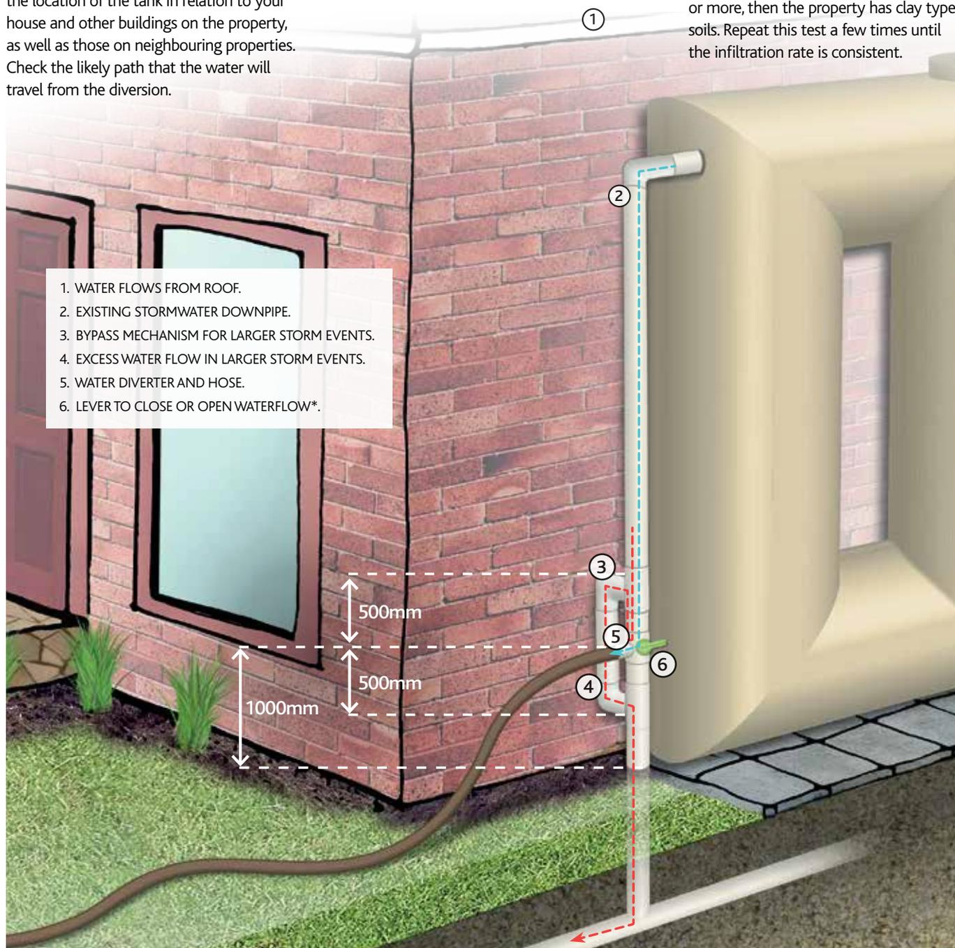
\* Diverter most effective when lever pushed closed
