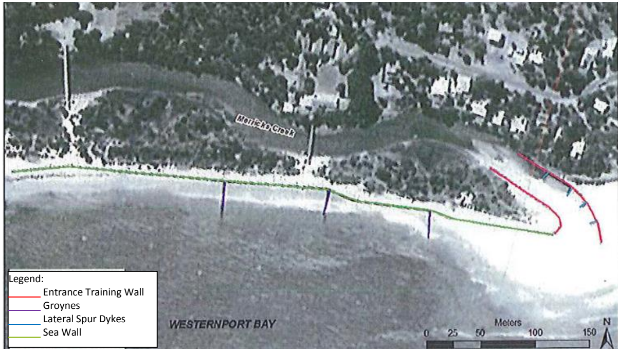
Figure 8. Works undertaken 1960-1975 – aerial photo ~1977 (Water Technology 2011) timber training wall shown in red and timber sea wall shown in green
