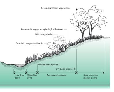
Figure 16 An example of a cross-section showing zones according to moisture gradients along the stream bank and verge.
