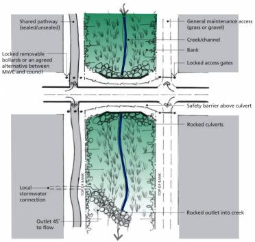
**Figure 22** An example of a constructed waterway showing shared pathway on one side and general maintenance access on the other. A minimum offset of 5 m from the top of the bank is required.
