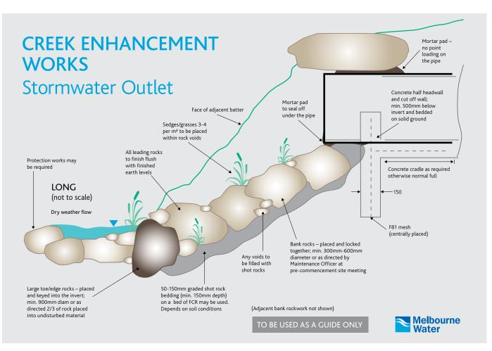
Figure 14 Stormwater outlet design. (Note that this figure is to be used as a guide only as the size of the rock and extent of the rock beaching will depend on pipe size, creek profile and expected discharge from the outlet.)
