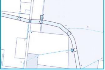
GREENFIELD DEVELOPMENT SITE Developer A Stage 2 Invert levels to match upstream property Developer B DEVELOPMENT Stage 1 SITE WITHIN THE DEVELOPMENT SERVICES SCHEME HYDRAULIC RESERVE WIDTH OVERALL RESERVE WIDTH Invert levels down stream Developer C to achieve free Stage 3 draining outlet Negotiate works in adjacent downstream property to **RURAL / FUTURE** enable free **DEVELOPMENT SITE** draining outlet
