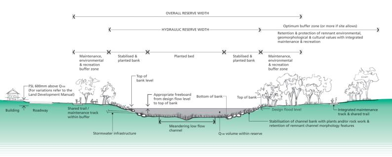
**Figure 23** Contemporary waterway design showing the 100-year event contained within the main waterway in urban development areas. The hydraulic and overall reserve width will vary for each waterway.
