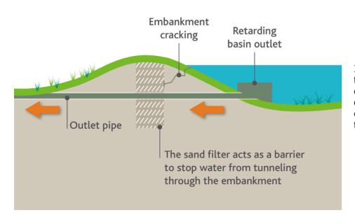
Installing a sand filter or filter trench can prevent water destabilising the embankment by flowing through it.
