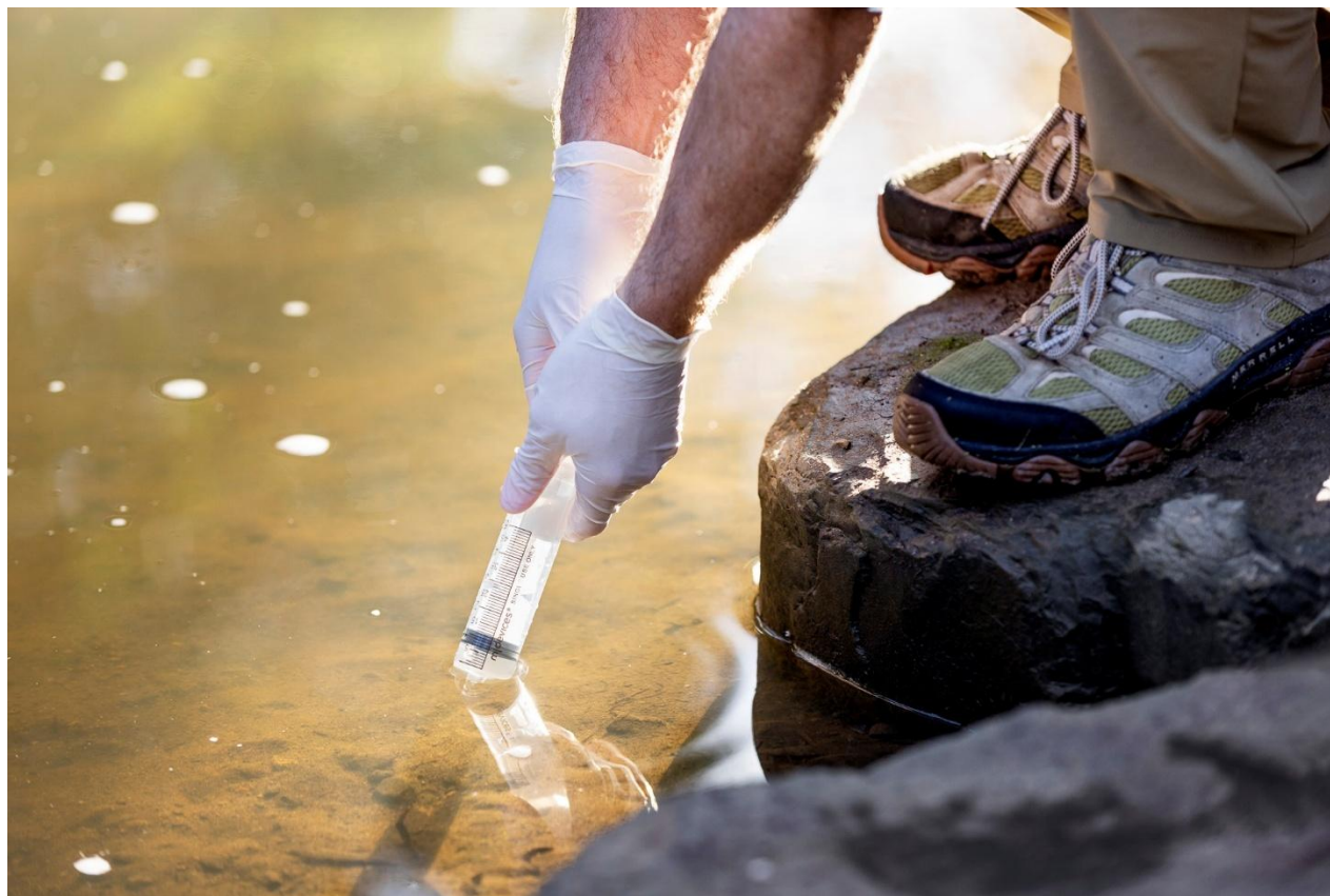
Figure 4. Collecting a water sample to enable the filtration of DNA for later analysis in the lab. Photo courtesy of EnviroDNA.
