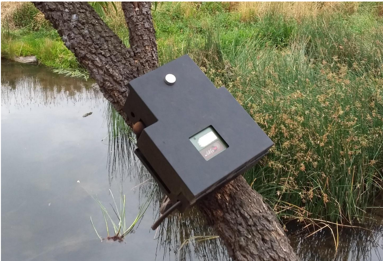
Figure 3. Song Meter SM4 (Wildlife Acoustics) secured to a branch overhanging a creek pool. Photo courtesy of Brendan Casey.
