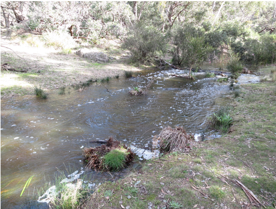
Figure 5-12 Photo of 30 ML/day at cross section 6 wetting the low edge of the bench
