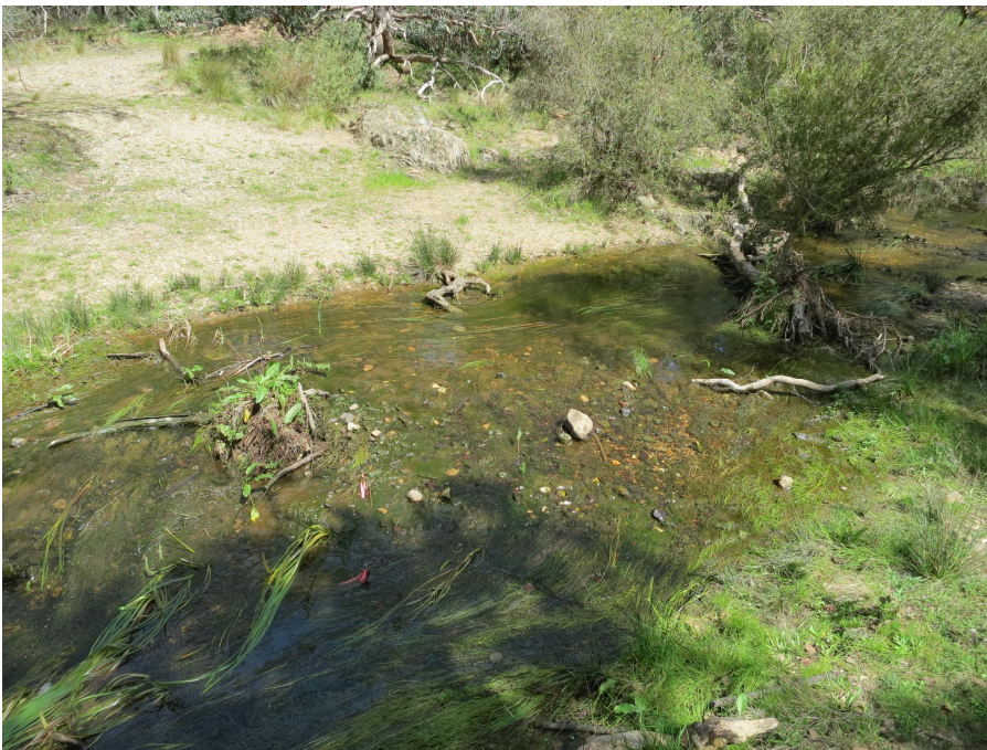
Figure 5-10 Photo of cross section 6, the shallowest cross section within the flows site, showing 1 ML/day. The low flow recommended will produce a larger wetted area.
