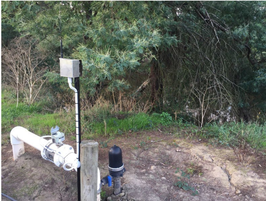
Figure 3: Full flowing pipe meter with telemetry transmitter
