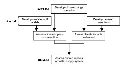
Figure 10: Modelling process flowchart for water supply case study
