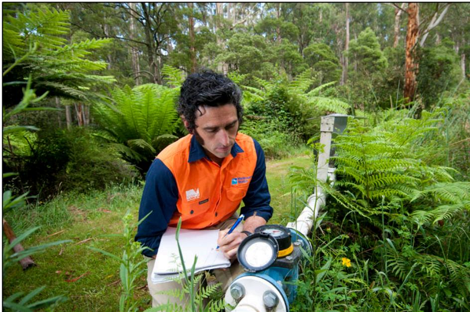
*Irrigation meter being read by Melbourne Water*
