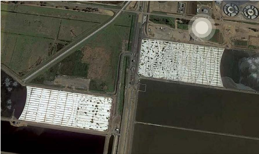
Aerial view of the two covered anaerobic lagoons at the Western Treatment Plant
