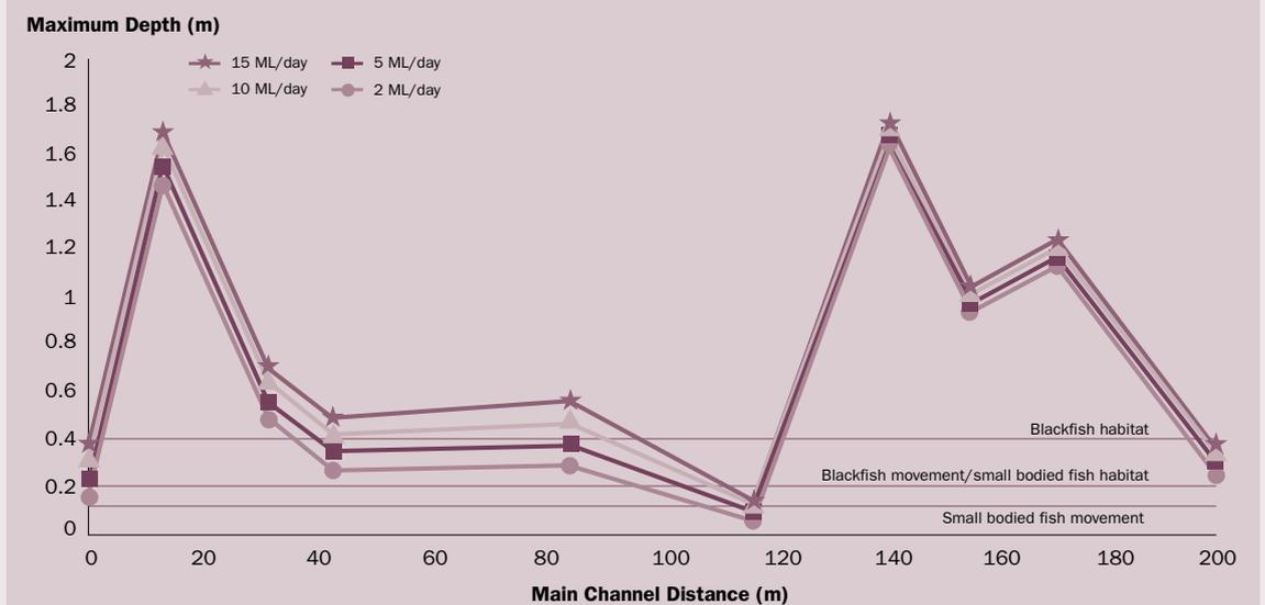
Figure 7 Pauls Creek Water depths at various flow rates showing ecologically important depths
