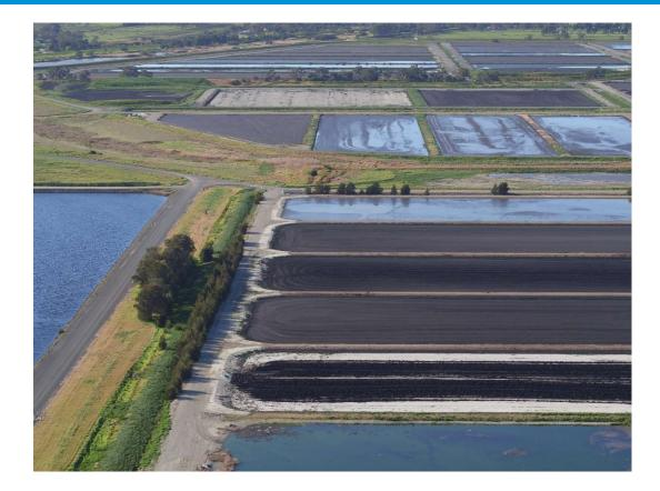
Digested sludge drying pans
