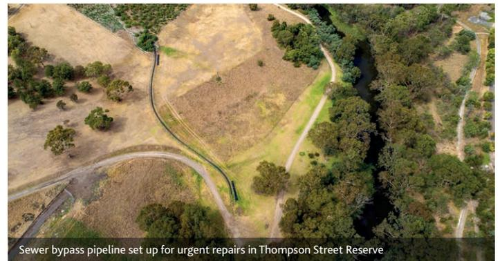
Sewer bypass pipeline set up for urgent repairs in Thompson Street Reserve
