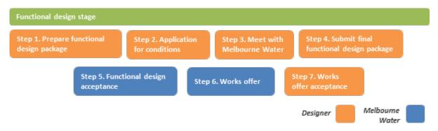
Figure 3 Steps in the functional design phase
