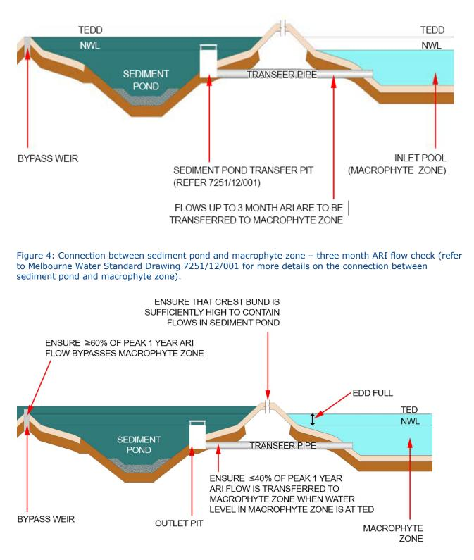
Figure 5: Figure 6 Connection between sediment pond and macrophyte zone – one year ARI flow check (Refer to Melbourne Water Standard Drawings 7251/12/001 for more details on the connection between sediment pond and macrophyte zone).
