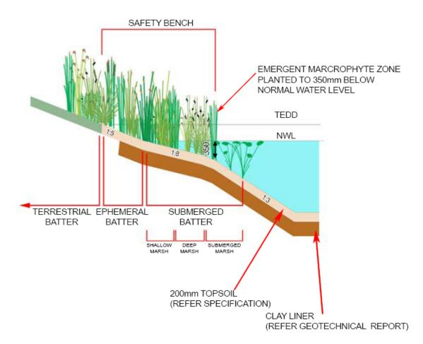
Figure 6: Indicative cross-section of vegetated wetland edge with safety bench (Refer to Melbourne Water Standard Drawing <u>7251/12/010</u> for more details).
