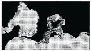
Figure 4.7. Bathymetry of Western Port used in numerical modelling for the Better Bays and Waterways program, 2004-08. The black contour line marks 0 m, or lowest astronomical tide used as chart datum. (Source: Harrison *et al.* 2011a)
