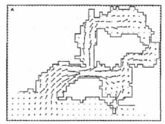
Figure 4.6 Two-dimensional nested model of localised Bass Strait hydrodynamics. (Source: Black and Hatton, 1994).
