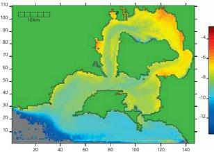
Figure 4.46 Mean concentration (kg/m<sup>3</sup>) of toxicants from freshwater input, 2004. Levels are higher near the Bunyip, Lang Lang, and Corinella segment in the east. (Adapted from Harrison *et al.* 2011b.) Tox log (Mean Conc) 2004
