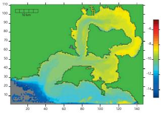
Figure 4.48 Total suspended solids (kg/m<sup>3</sup>) with wave mixing and sediment resuspension included. (Adapted from Lee *et al.* 2011.)
