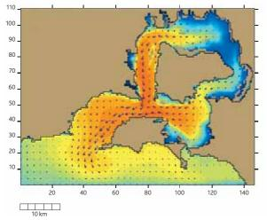
Figure 4.55 Distribution of Western Port T90 residence times (in days) throughout the 2004 (left panel) and 2030 (right panel) flushing simulations. Simulations based on the flushing of a conservative tracer from the Port. (Source: ASR, unpubl. data).
