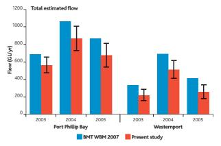
Figure 4.59 WaterCAST catchment model showing good agreement with measurements. (Source: Stewart *et al.* 2010.)
