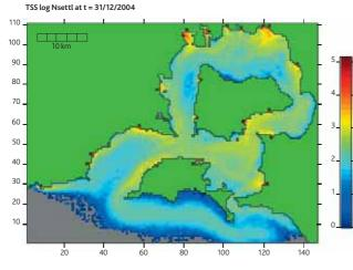
Figure 4.47 Mean concentration (kg/m<sup>3</sup>) of nitrogen (all types) from freshwater inputs in 2004, plotted on a logarithmic scale. (Adapted from Harrison *et al.* 2011b.)
