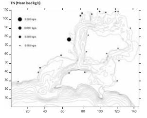
Figure 4.43 Mean integrated number of visits to cells by suspended solids (mud, 6 phi) delivered by rivers in 2004, plotted on a logarithmic scale. A larger integrated number count suggests increased availability of mud in suspension as well as indicating major transport routes. (Adapted from Harrison *et al.* 2011b.)
