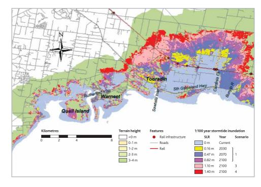
Figure 4.52. Land vulnerable to inundation during a 1 in 100 year storm tide under current climate conditions and various scenarios of future sea level rise for the Tooradin region. (Adapted from McInnes *et al.* 2009a.)
