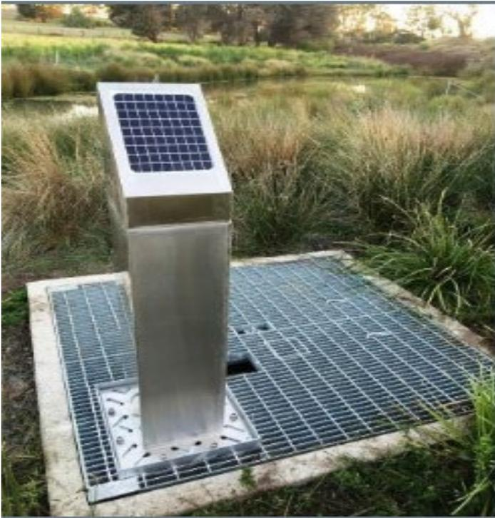
Figure 3: Hydraulic level sensor & data logger
