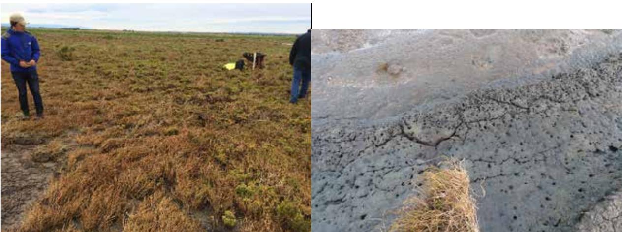
Figure 31 Left: Vegetation density affected by wave inundation behind the crenulation section. Right: Looking downwards showing tension cracks running along the top of the lower bank adjacent to the headland at the southern end of the site.
