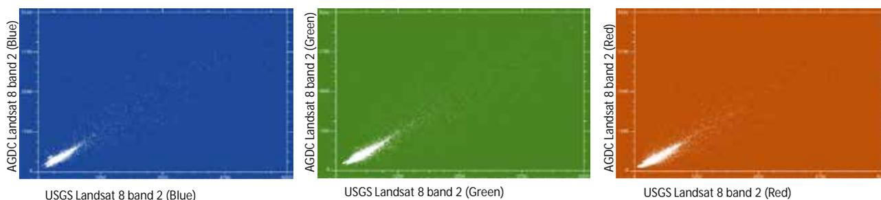
**Figure 58: The comparison between the surface reflectance products produced by the AGDC (y-axis) and the USGS (x-axis) for the blue, green and red bands.**
