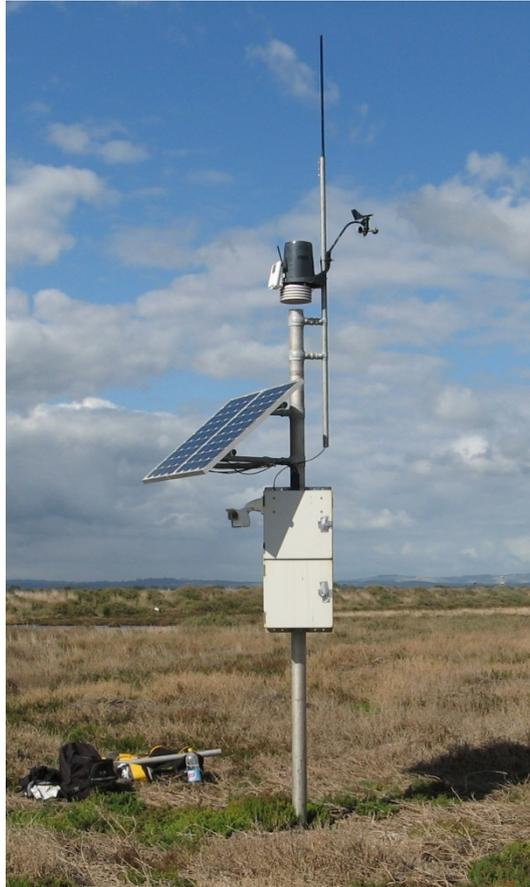
Figure 6. Monitoring camera, solar panels and weather station installed at the site.
