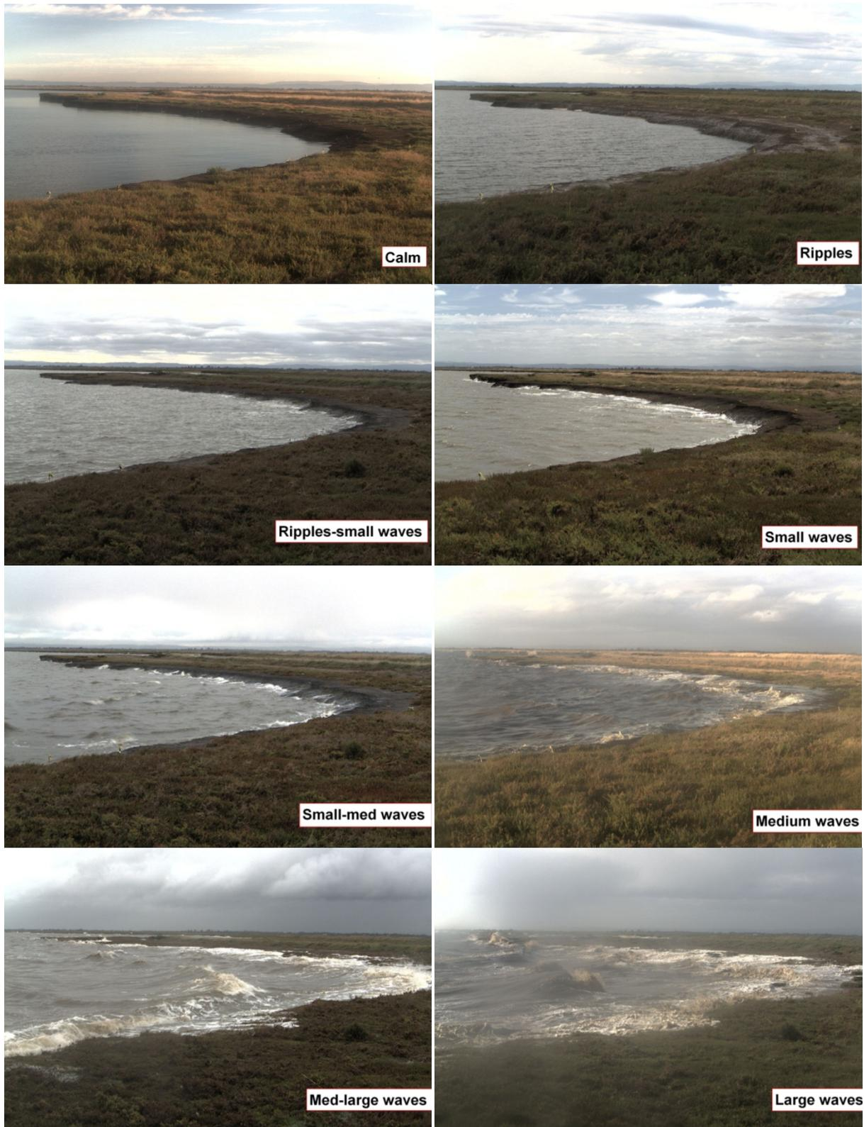
Figure 7. Examples of the classification system used to characterise the wave conditions during each high tide.
