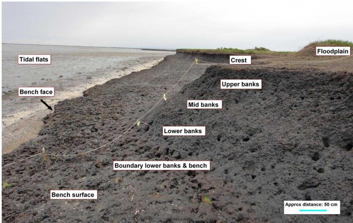
Figure 5. Example of one of the erosion pin transects, showing the geomorphic units identified. The units were also used to classify the heights reached during each high tide.
