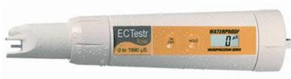
**IMPORTANT NOTES:** Pour water from your sample bottle into a rinsed beaker for testing. Insert only the tip of your EC meter into the water.
