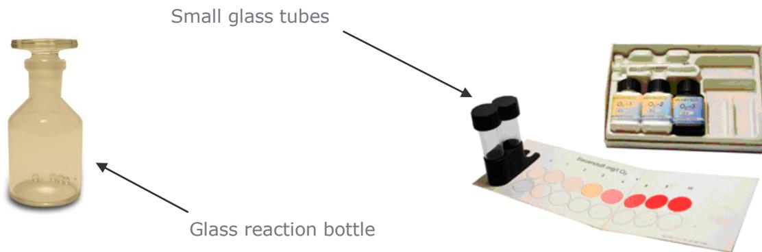
**IMPORTANT NOTES:** Wear gloves to undertake this test. The reaction takes place in the glass reaction bottle. Waste can be disposed of down a sink connected to the sewage system, with lots of water.
