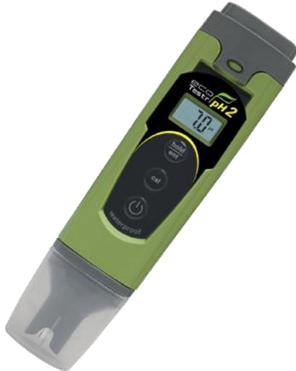
**IMPORTANT NOTES:** Pour water from your sample bottle into a rinsed beaker for testing. Insert only the tip of your pH meter into the water.
