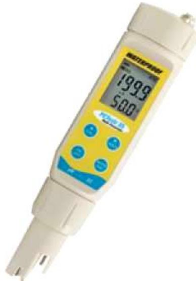
**IMPORTANT NOTES:** Pour water from your sample bottle into a rinsed beaker for testing. Insert only the tip of your EC meter into the water.
