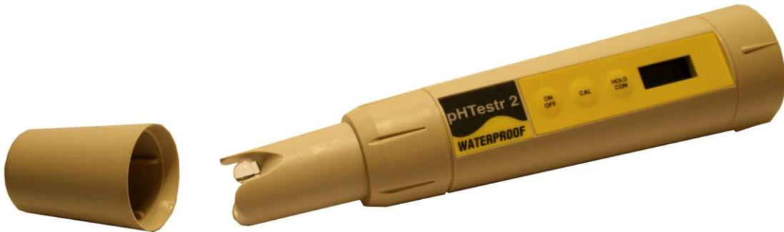
**IMPORTANT NOTES:** Pour water from your sample bottle into a rinsed beaker for testing. Insert only the tip of your pH meter into the water.
