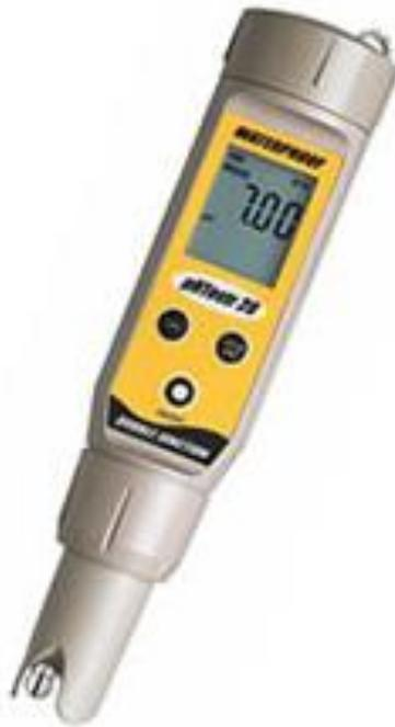
**IMPORTANT NOTES:** Pour water from your sample bottle into a rinsed beaker for testing. Insert only the tip of your pH meter into the water.
