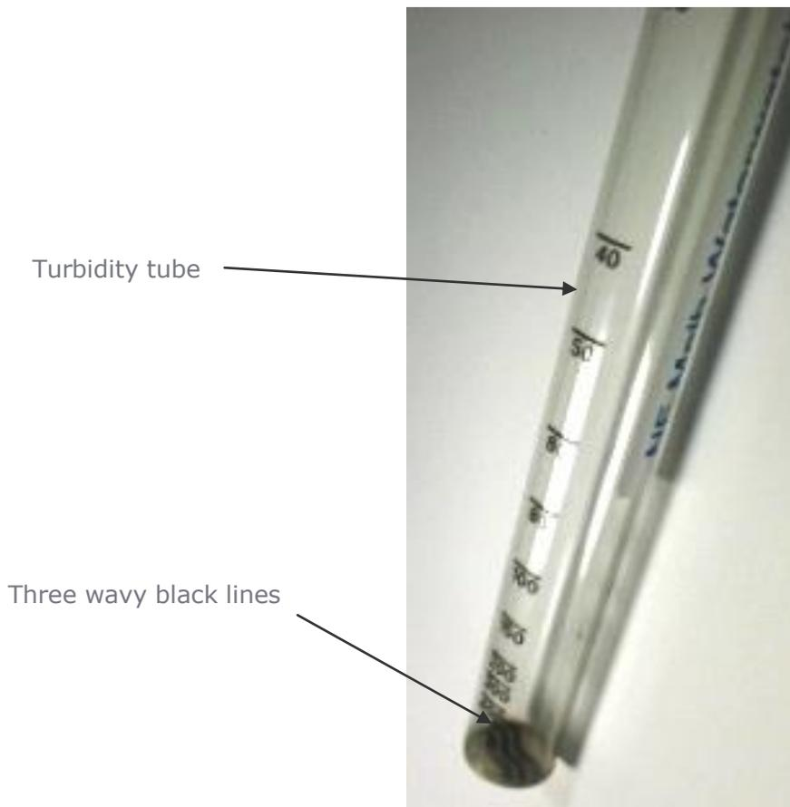
**IMPORTANT NOTE:** Stand in a shady place when viewing down the turbidity tube. Shake your sample before testing.
