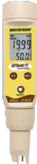
**IMPORTANT NOTES:** Pour water from your sample bottle into a rinsed beaker for testing. Insert only the tip of your EC meter into the water.
