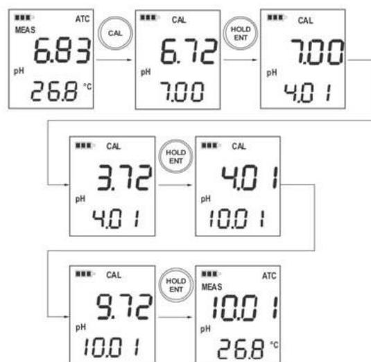
Figure 1: Eutech pH Testr10 Calibration
