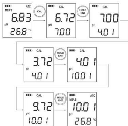
Figure 1: Eutech pH Testr10 Calibration
