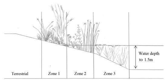
Figure 17 Conceptual cross section of the embankment for revegetating wetland environments, showing terrestrial vegetation and wetland vegetation zones 1, 2 and 3.
