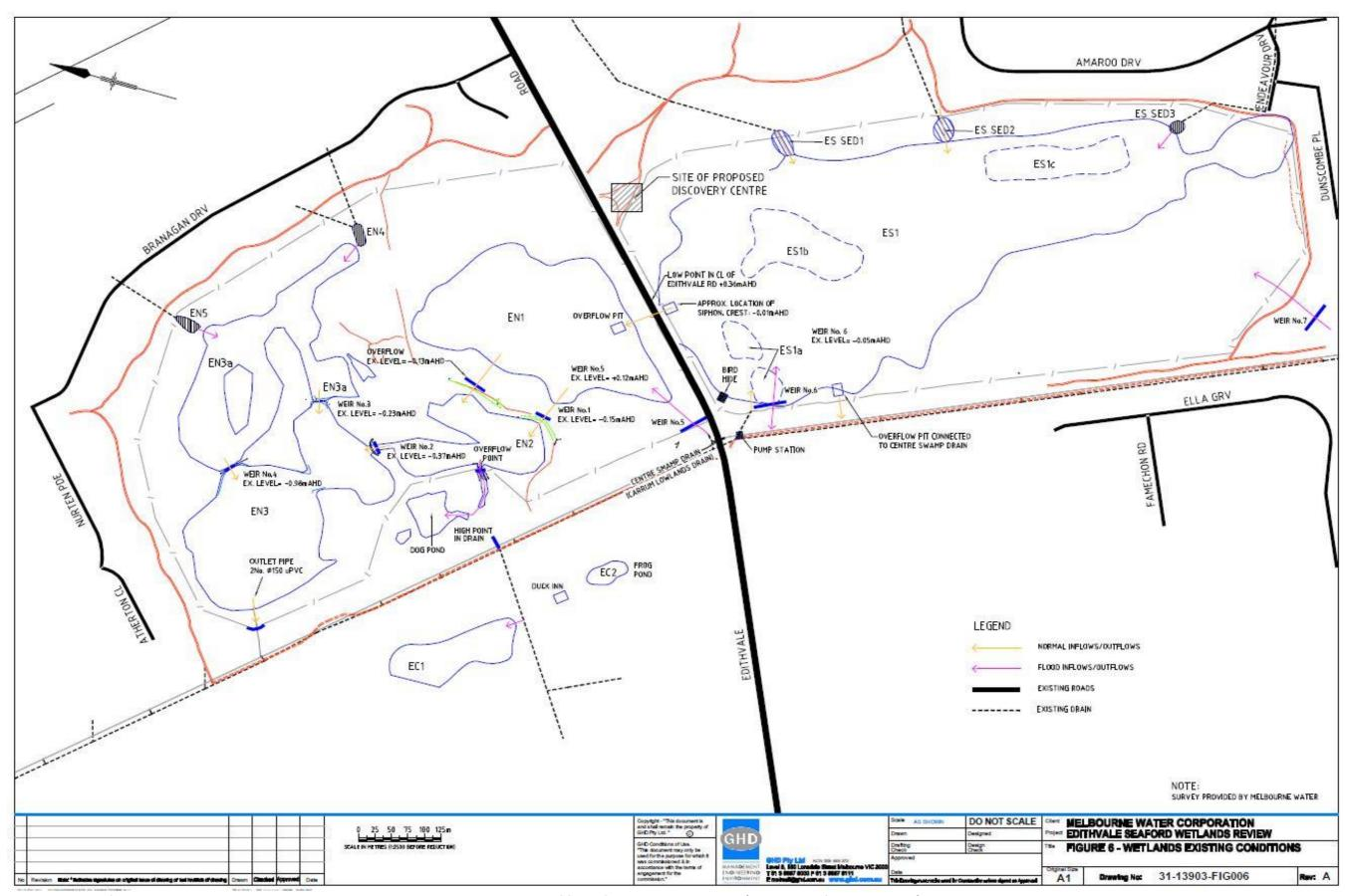
Figure 12Location of hydrological cells, drains, weirs and sedimentation ponds and direction of flows for Edithvale Wetlands (reproduced from GHD 2006).
