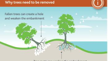
Tree roots can weaken the embankment increasing the risk of embankment failure
