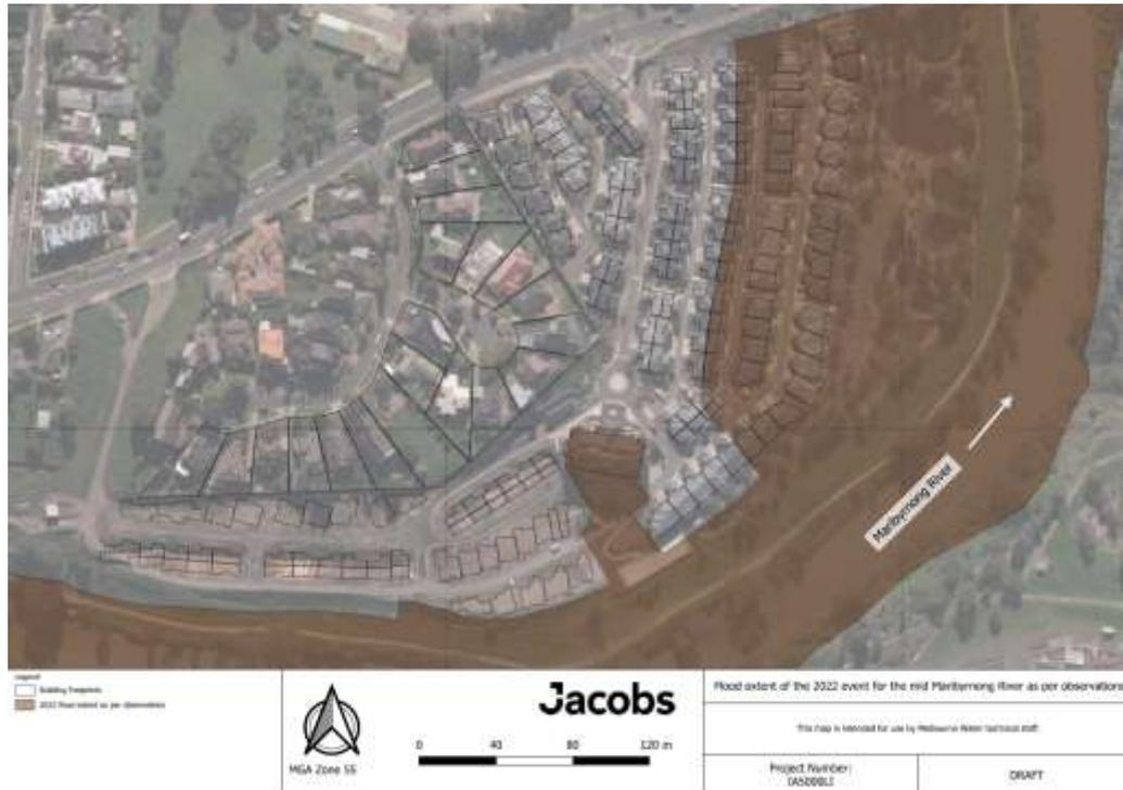
Figure 12: Estimated extent of inundation at Rivervue Retirement Village for the Flood Event. (Source: Jacobs 2023, Mid\_Maribyrnong\_2022\_Flood\_Extent\_Observations, provided by Melbourne Water in folder “1. Mapping”).
