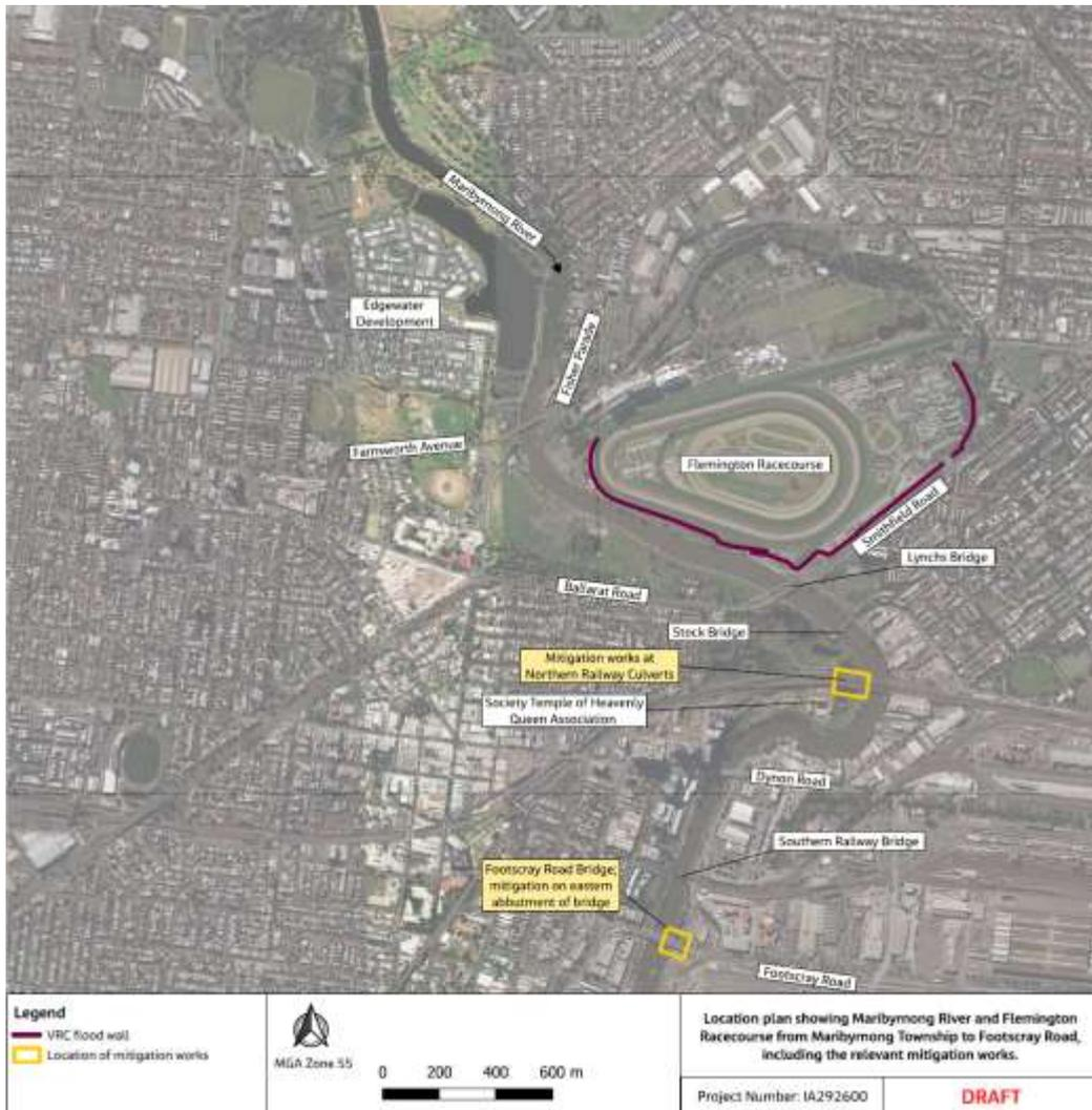
Figure 48: Location of Flemington Flood Wall and Associated Compensatory Works. (Source: Additional documents provided to IRP by Melbourne Water upon request, 5. Background Documents – Flemington Wall, File titled “Location\_plan\_map\_opt.pdf”).
