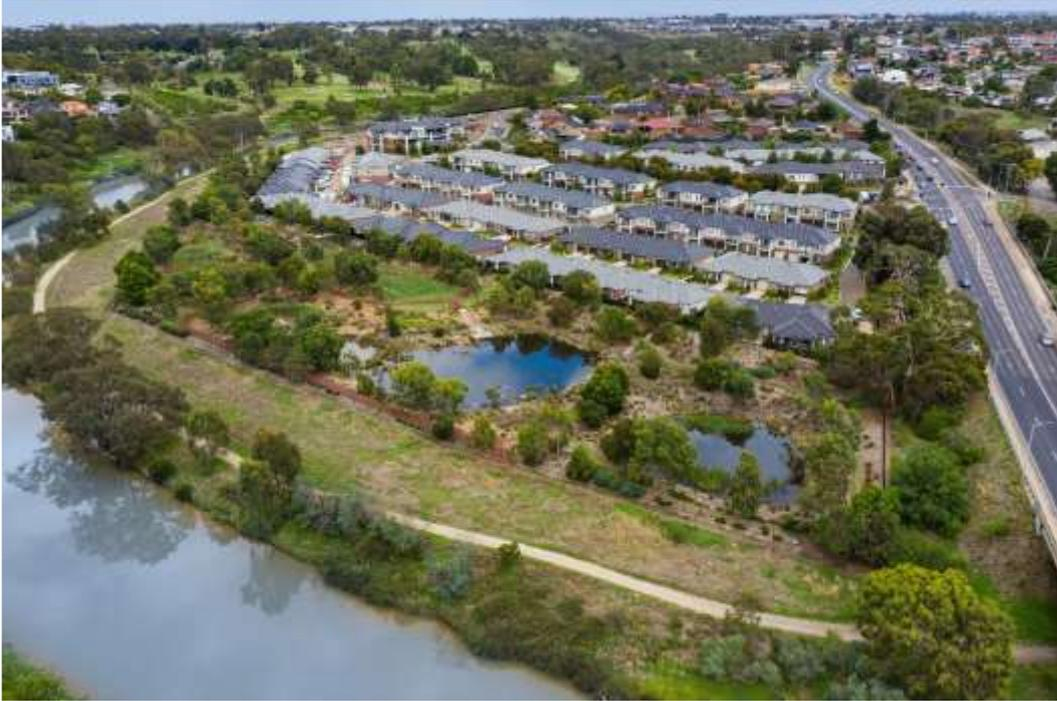
Figure 10: Photo of Rivervue Retirement Village (prior to the Flood Event), showing the constructed retarding basins in the area of the site close to the river corridor land. Canning Street is seen at the right of photo.
