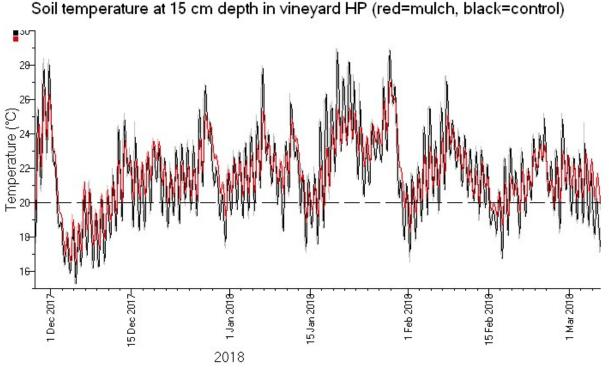
Figure 5: Hourly measurement of soil temperatures by Tinytag loggers in Pinot noir at Handpicked Wines
