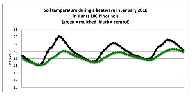
Figure 6: Soil temperatures at 15cm during a heatwave using Carta sense technology
