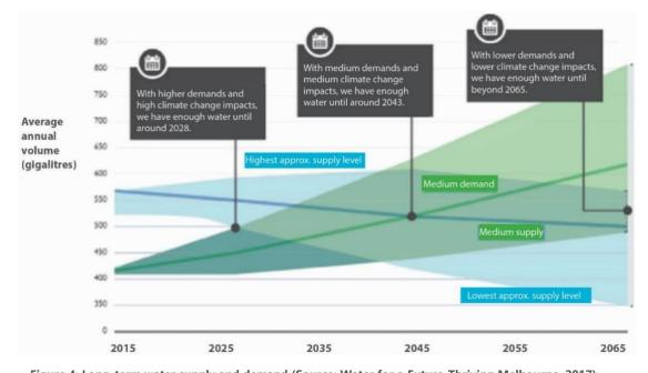
Figure 4: Long-term water supply and demand (Source: Water for a Future-Thriving Melbourne, 2017)
