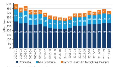
Figure 5: Melbourne's total water use by segment
