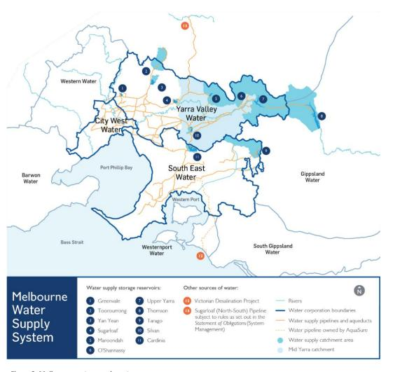
Figure 3: Melbourne water supply system
