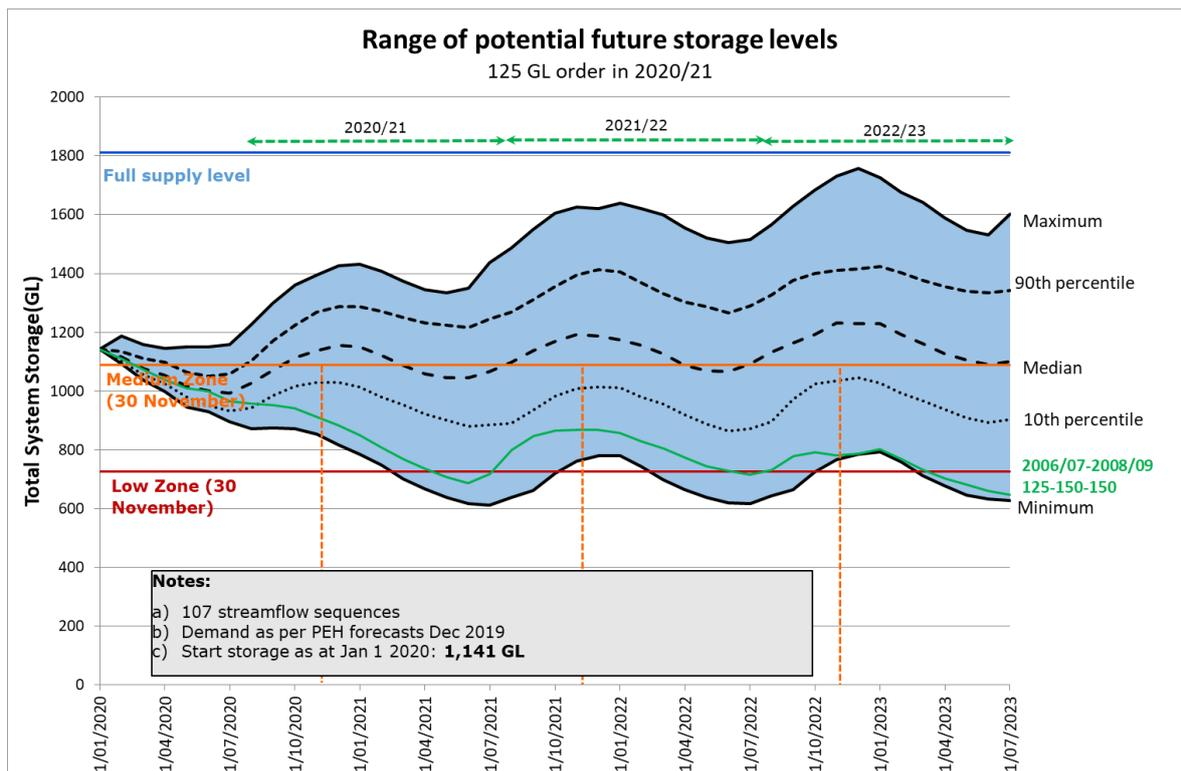
Figure 4: Modelled projection of potential future water storage levels assuming a 125 GL order in 2020/21
