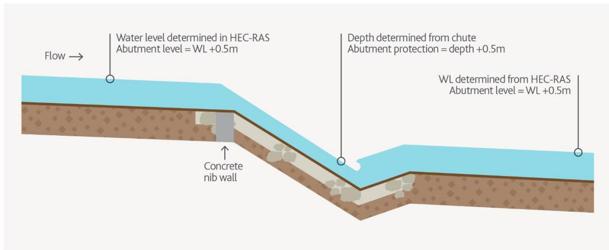
**Figure 57 - Schematic of a typical Chute**
