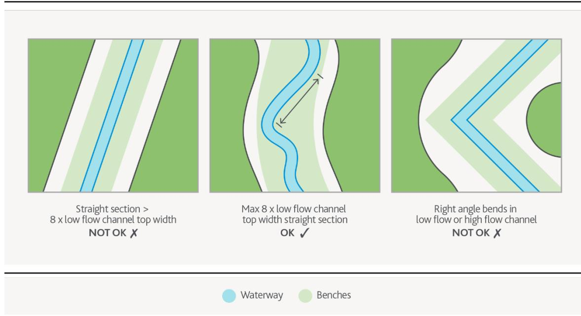
Figure 36 - Bend sharpness acceptable limits for compound waterways
