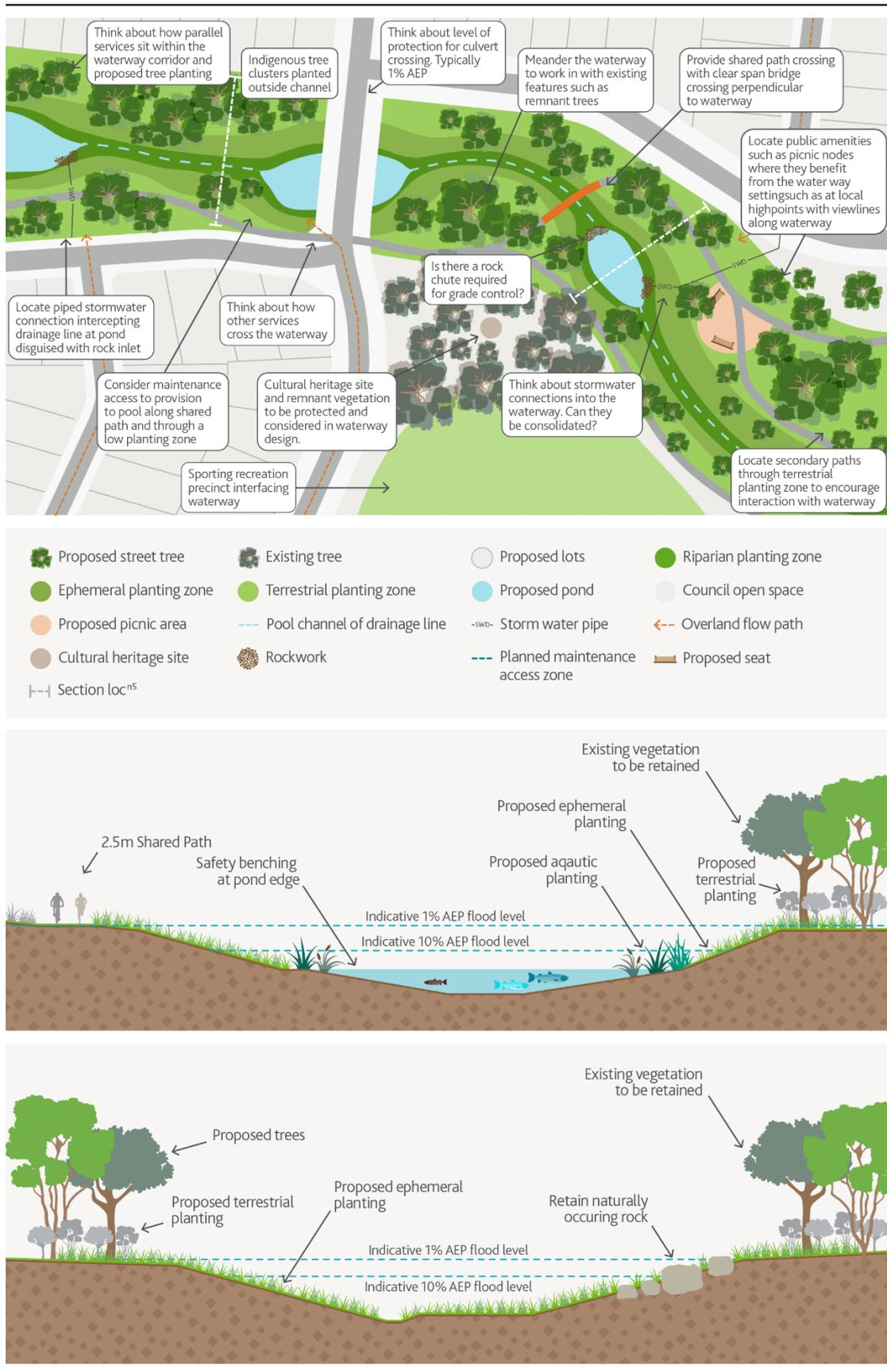
Figure 32 – Example constructed waterways concept design
