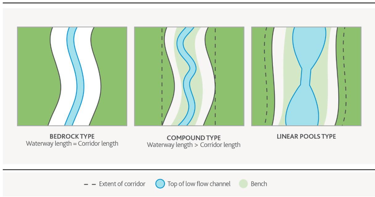
Figure 30 - Examples of the three constructed waterway types
