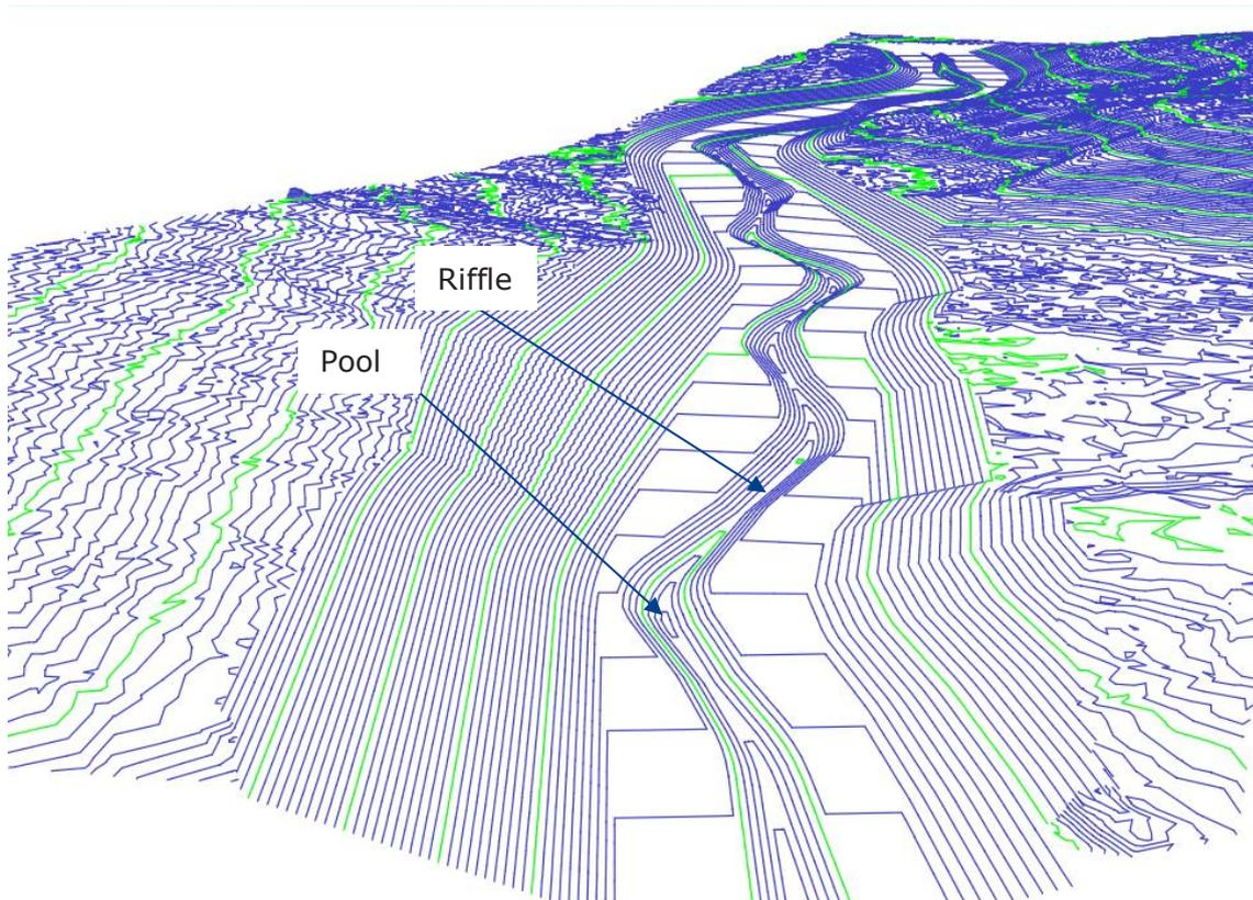
Figure 65 - Example terrain model of compound type waterway showing platform variation. Pools and riffles have been introduced at meander bends in the low flow channel
