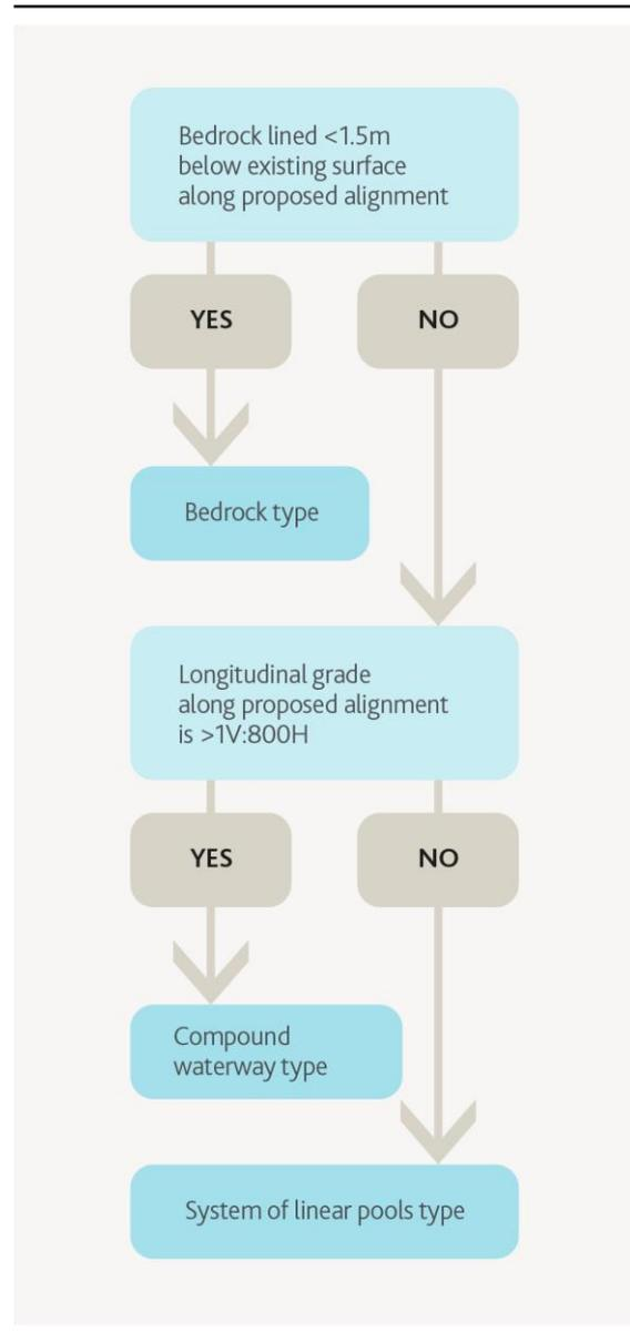
Figure 31 - Constructed waterway type decision tree
