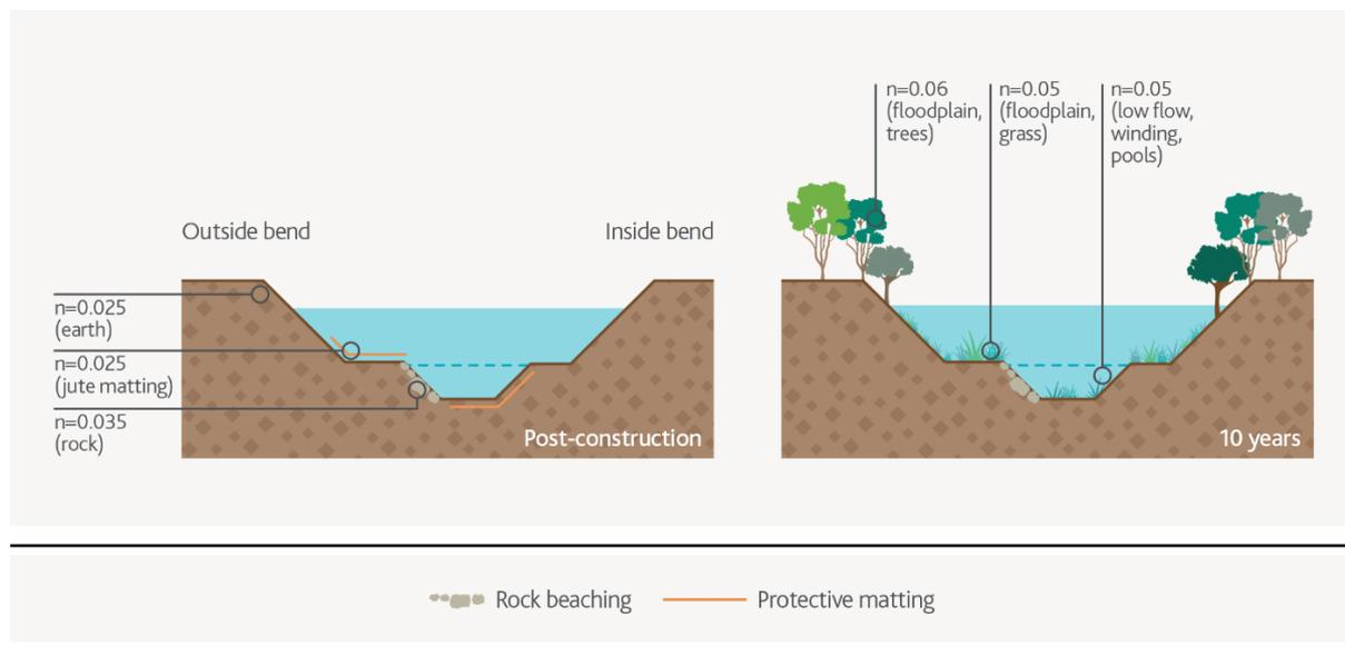
Figure 45 - Waterway corridor showing regions of similar vegetation species/hydraulic roughness in the immediate post-construction period when mature condition are reached (10 years plus)<sup>4</sup>
