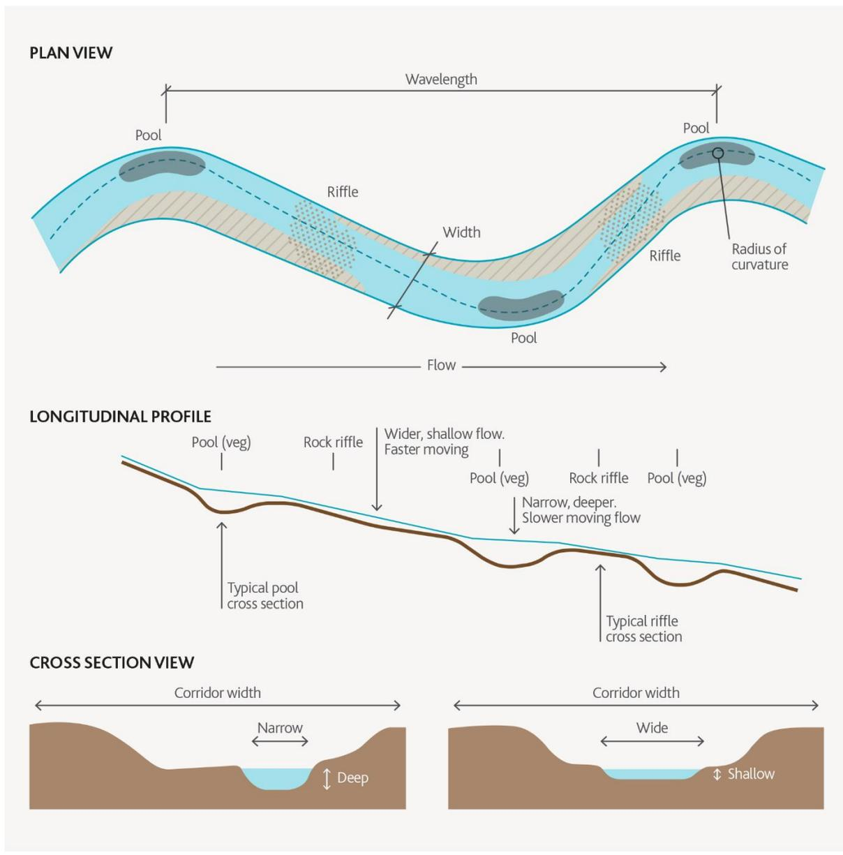
Figure 60 - Idealised pool-riffle sequence
