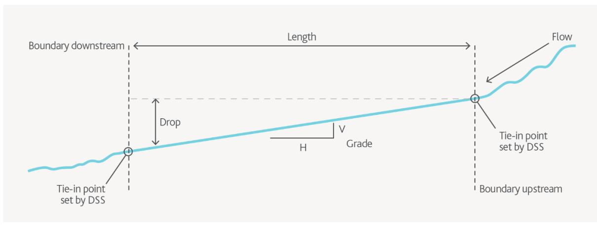
Figure 38 - Example calculation of channel slope
