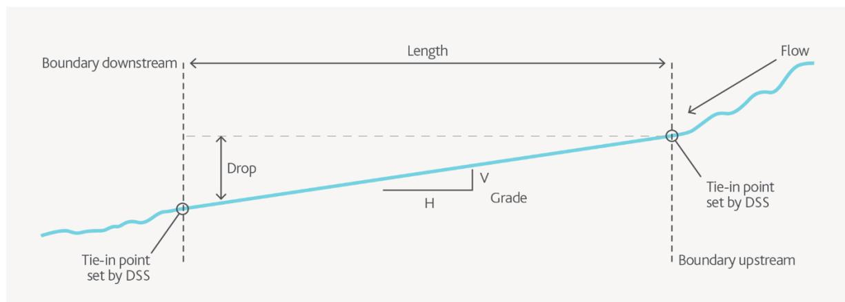
**Figure 27 - Parameters used to determine the longitudinal bed grade of a waterway**
