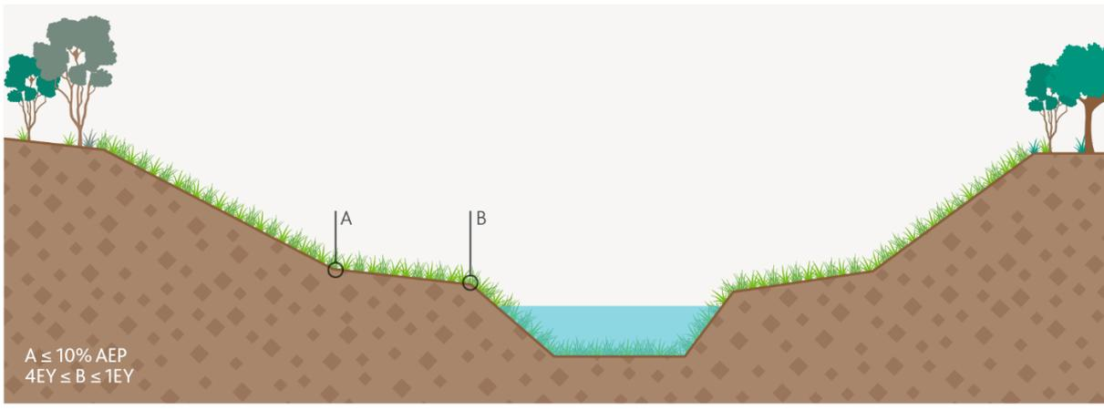
Figure 62 – Example cross-section illustrating the bench design criteria
