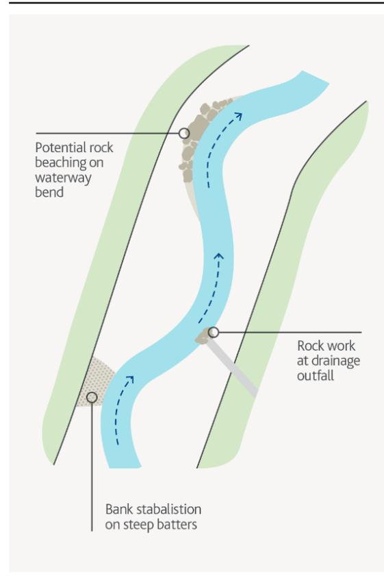
Figure 59 - Typical applications of rock beaching
