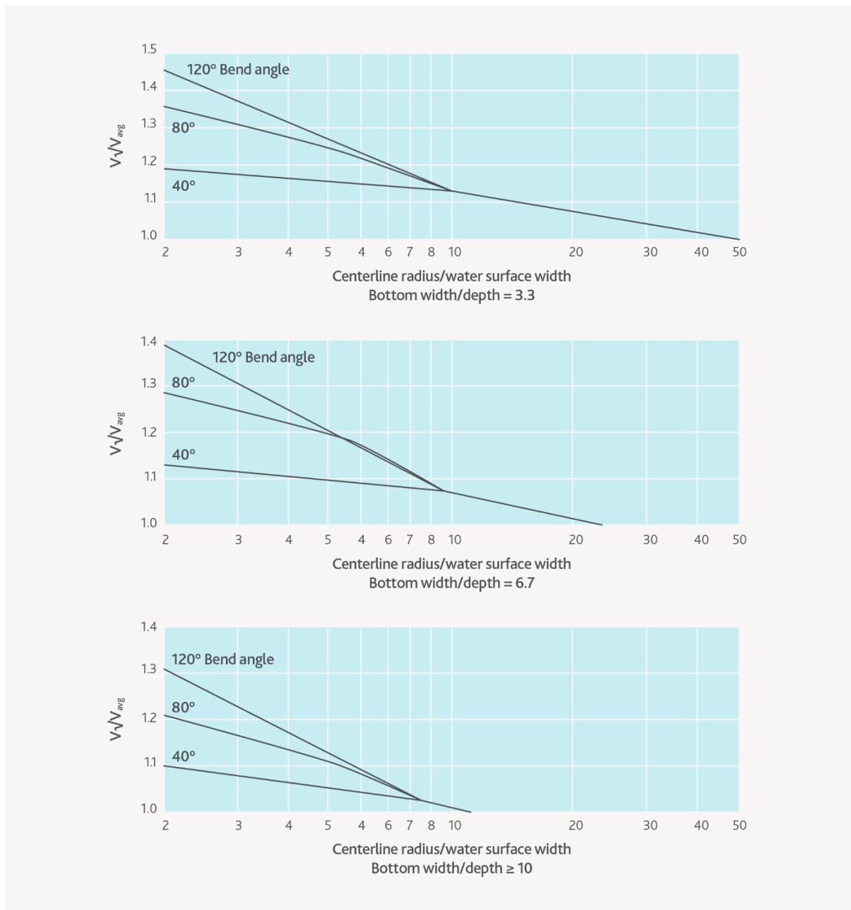
Figure 53 - Applied maximum velocity on bed and banks of trapezoidal channels in a curved reach (from NRCS 2007), where  $V_{ss}$  is depth-average velocity at 20% of slope length up from toes, maximum value in bend. Curves based on STREMR model (Bernard 1993),  $V_{avg} = 6\text{ft/s}$ , 1:3H side slopes.  $N = 0.038$ , 15ft depth
