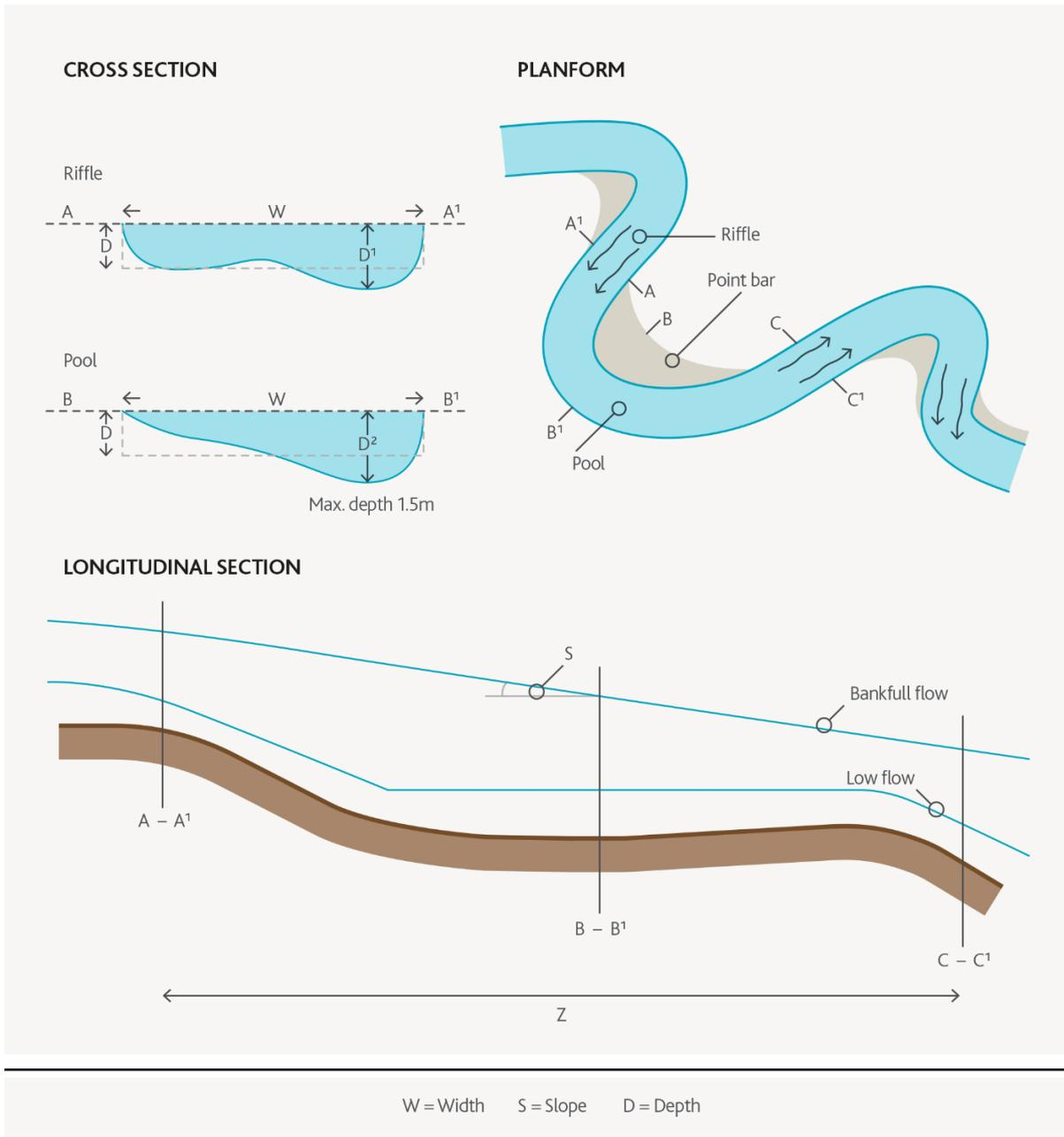
Figure 13 – A typical pool-riffle sequence<sup>1</sup>
