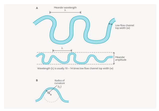
Figure 10 - Aspects of meander geometry (a) Meander wavelength. (b) Radius of curvature
