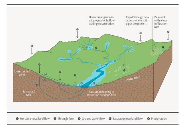
Figure 3 - Hydrologic pathways generating flow in an undeveloped catchment
