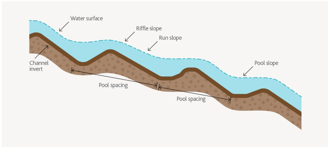
Figure 11 – Example waterway long-section (longitudinal profile)
