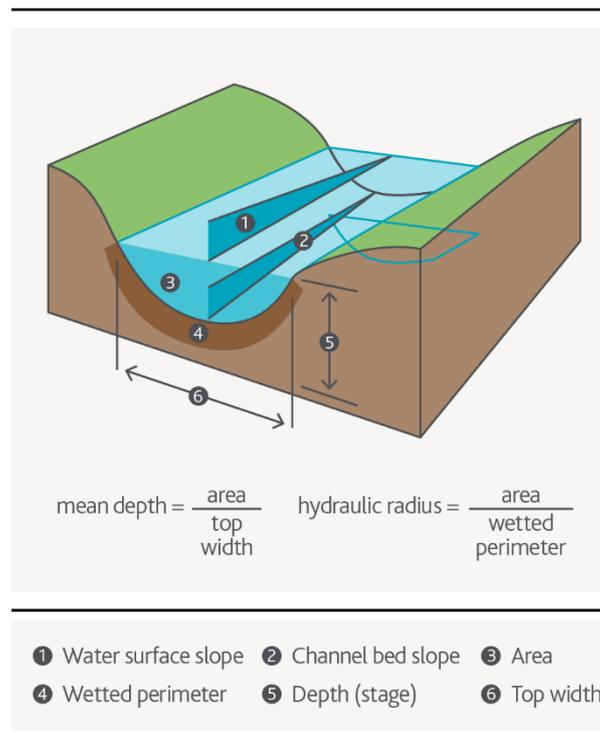
Figure 6 - Illustration of parameters in the Manning equation
