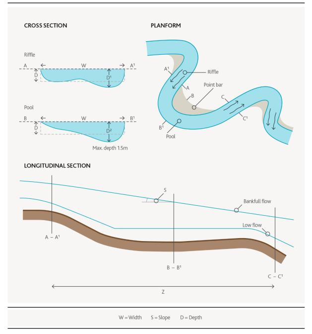
Figure 13 – A typical pool-riffle sequence<sup>1</sup>
