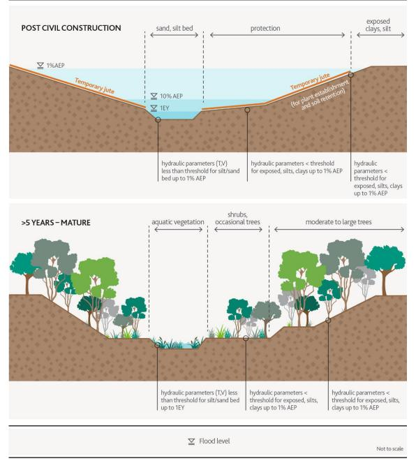
Figure 1 - Spatial and temporal variability of waterways – implications for the threshold design approach (T=shear stress, V=velocity)
