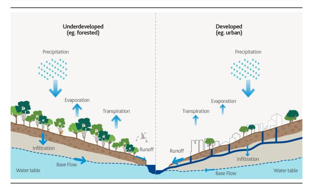
Figure 4 - Comparison of hydrologic pathways generating waterway flow between a developed and an undeveloped catchment.
