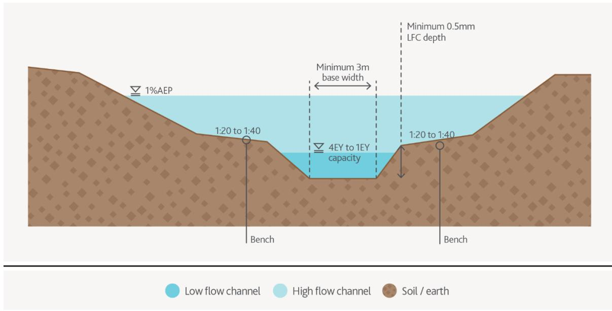
Figure 12 - Typical compound waterway section example
