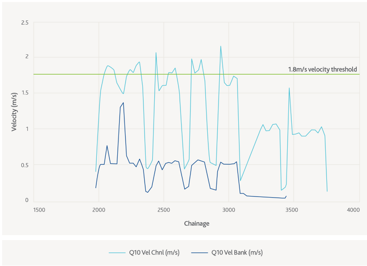
Figure 54 – Post-construction maximum velocity along the waterway for a 10%AEP event
