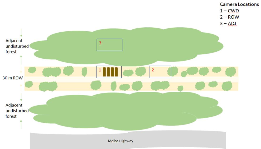
**Figure 2 Habitat linkage camera set up (one set)**
