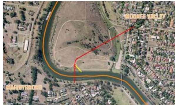
Figure 1 – Area of works showing existing north western sewer main in red and intended structure in yellow
